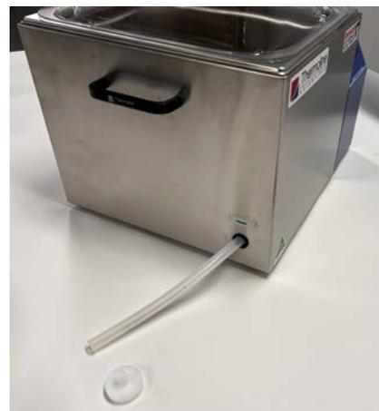
To drain the bath simply find the drain located on the side of the bath and pull it out (exposing the hose). You can then remove the plug to drain the water.
