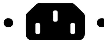
Fig 2. 10 amp male IEC socket
