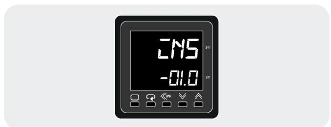
Use the **UP** or **DOWN** button to adjust the sensor correction.
