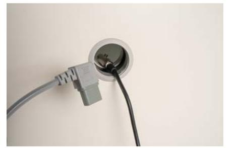
Power down the TMLR-200 before installing the TPS-18. Plug the power lead into the port on the side of the TMLR-200 and feed both leads through the 54mm port hole. Using a trolley, bring the TPS-18 close to the open door of the TMLR-200 and connect the power and BMS leads. Carefully slide the TPS-18 into the TMLR-200.
