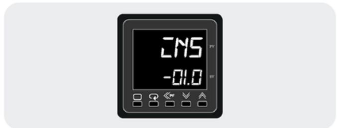
Use the **UP** or **DOWN** button to adjust the sensor correction. After this, allow the digit to stop flashing and the screen will display the adjusted value. Press **PAGE** to exit back to the main screen.
