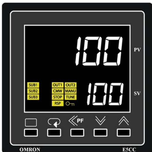
**Note:** Limited access to the controller is available. The operator has access to alter the temperature set point and parameters used for calibration purposes only.
