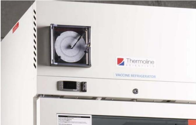
A circular chart recorder can be factory fitted as an optional extra. The recorder has a seven day chart with a battery back-up that will keep the chart running for at least 24 hours in the event of a power failure.
