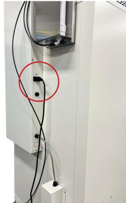
Fig 3. 15A/230V IEC socket location.
