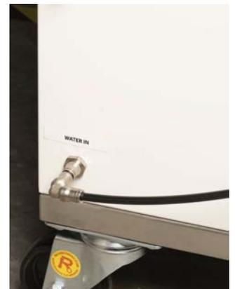
Fig 4. Connecting to the cabinet water inlet.
