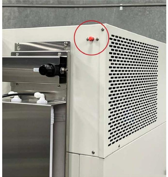
**Fig 2. Refrigeration safety pressure switch location**
