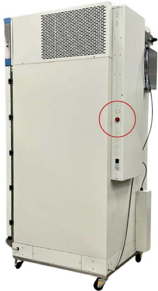
The temperature controller on the Envirotherm cabinet is a STAR X touchscreen. The Thermoline STAR X has been designed and configured to provide ease of use and a suitable level of security. The STAR X has a unique identifier that allows traceability back to the instrument.
