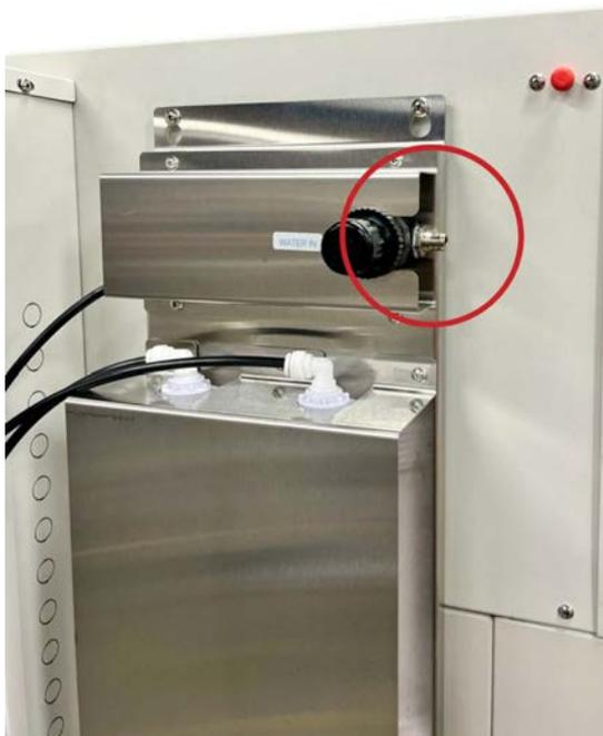
Fig 6. Water Pressure Regulator Connection
