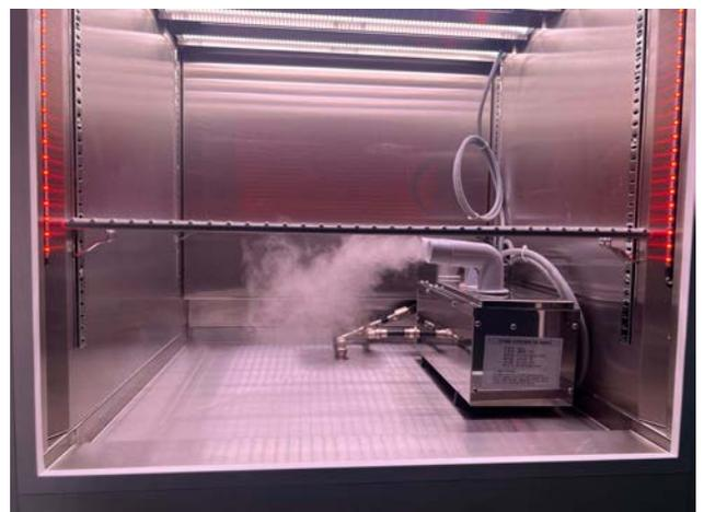
**Fig 4. Humidifier in place**
