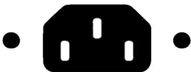
Fig 2. 10 Amp IEC socket
