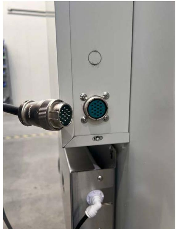
**Fig 3. Humidifier power connection**
