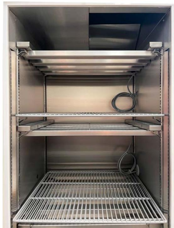
Shelf lights installed with power cables going through the 54 mm port holes.
