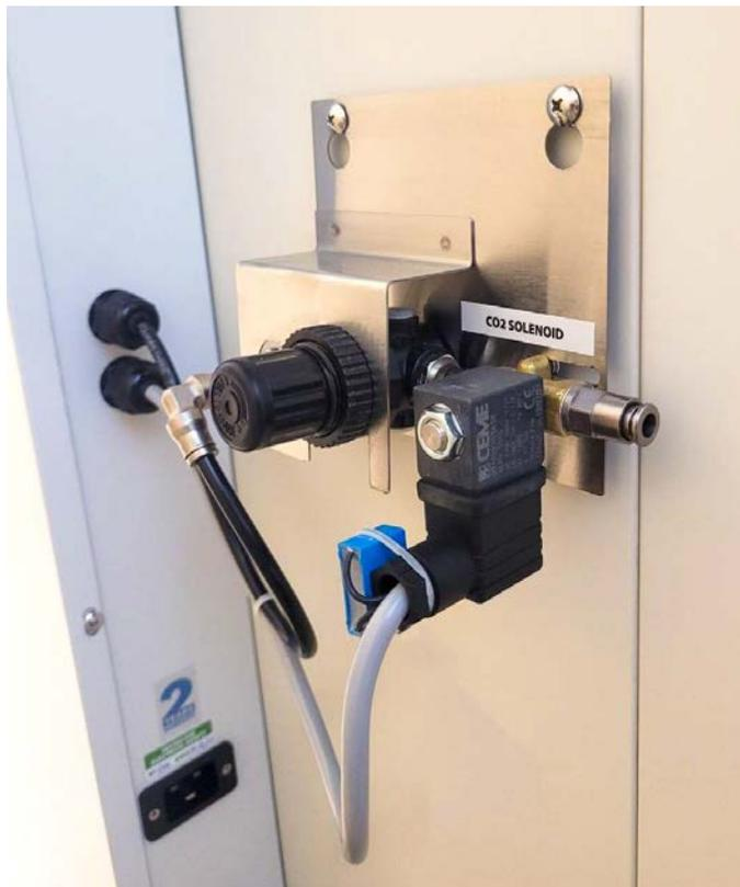
Fig 1. CO<sub>2</sub> connection
