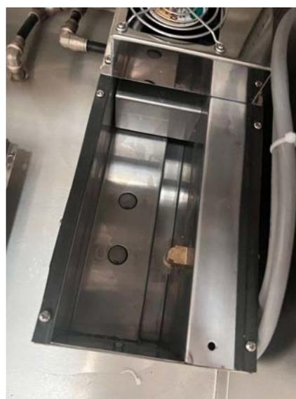
Once the water is drained, the nebuliser can be inspected (two small discs). The lid is held in place by four screws. There is often a small black dot at the centre. This is nothing to be concerned about and will not be able to be removed without causing damage. The nebuliser can be flushed with clean water if needed. Replace the lid once clean, and close the drain valve. With the water supply turned back on, the humidifier will refill once the Climatron is turned back on.
