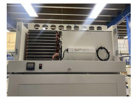
Pull the panel forward free of the blocks. This will allow you to access the controller
