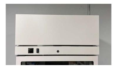
With the finger guard now in place, you can reinstall the front panel. Place the panel slightly above it's final position matching the rectangular holes with the locating blocks.
