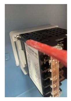
Once the wires have been removed, loosen the screws holding the white controller fixing bracket in place. The screws don't need to be completely removed from the bracket. Once loosened slide the bracket off. Once the bracket has been removed from the controller you can slide the controller out through the front face plate.
