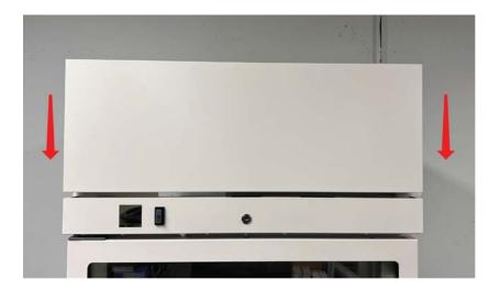
Push the panel forward onto the blocks then slide it down to lock into place.
