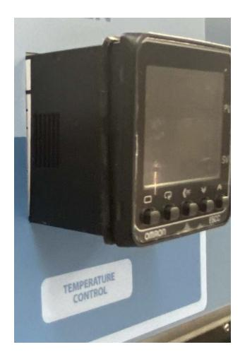
Slide the new controller into the front panel of the incubator.
