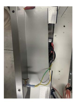
First remove the two screws holding the finger plate in place. Put this to one side leaving the earth wire attached. This will allow access to the rear of the Omron E5CC controller.
