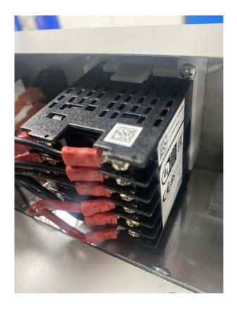
Disconnect the wires at the back of the controller, noting where each wire is located. Please note the included electrical diagram for wire connection locations.
