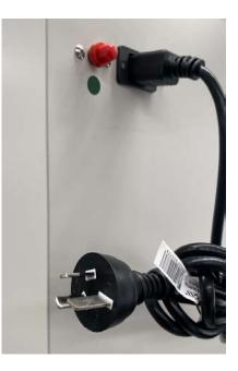
Turn off and disconnect oven from power. Allow the incubator to cool.
