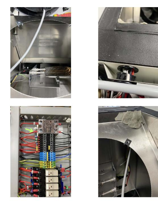
Thread the heating element wires through the bracket on the cabinet wall remembering to ensure the lock nuts are put over the wires at the correct locations to hold the element in the bracket. Next, thread the wires through the back wall. Attach the red wire to the relay using an appropriate fork terminal. Attach the neutral wire back into the terminal block. A wiring diagram is supplied on the next page for reference.
