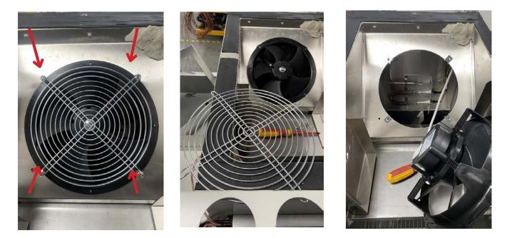
Remove the screws holding fan and protector in place First remove the fan protector and next, gently pull the fan assembly forward to reveal the heating element.
