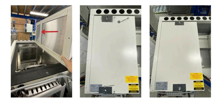
Replace the lid to the conditioning duct and reattach it with the screws removed earlier.
