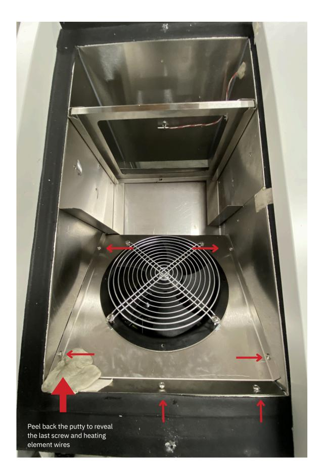
**Please note**: Another option to access the heating element is to remove putty and then remove the screws holding the fan motor plate in place allowing you to tilt it forward to access the heating element.
