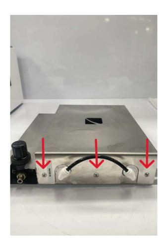
Remove the six screws on either side of the filter pack and lift off the front plate. Disconnect the hose running from the pressure reduction valve to the top filter (shown below with the red arrow). You can now remove the old filters. Note: You don't need to remove the hose running between the filters as a new one is supplied.
