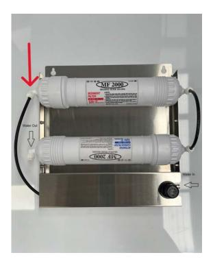
Place the new filters in the filter tray as shown above. Please ensure that the Activated carbon filter is placed closest to the black pressure regulator and the sediment filter is the furthest away. When installed like this the hose connecting the filters will be on the pressure regulator side of the filter pack. Reconnect the hose from the pressure regulator to the sediment filter inlet as shown.
