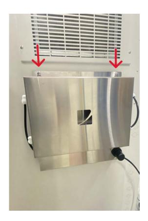
Put the cover back in place and reinstall the six fixing screws. Take the filter pack and hang it back into position. Once the filter pack is in place, the feed water can be connected water inlet on the pressure regulator and the feed to cabinet can be connected to the outlet of the filter back using the push-fit connectors.
