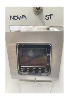
The two supplied metal plates slide over the Omron controller to sandwich the front panel where the previous Nova controller was housed to hold the new controller in place. Before inserting the Omron controller, take one of the metal face plates and slide it onto the back of the controller. With the first plate in place, slide the controller through the front panel.
