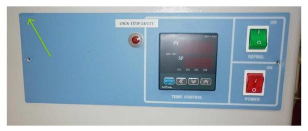
Undo the two screws holding the face plate in place (Red Arrows) and then lever the face plate forward from the corner (Green Arrow) to access the controller.
