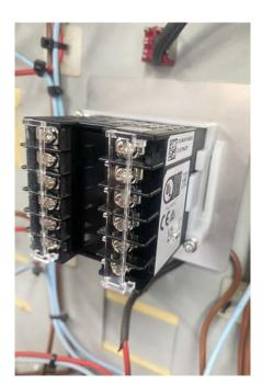
Slide the other faceplate on the back of the controller, so the wall of the incubator is sandwiched between the two supplied metal face plates. Next slide the white Omron fixing clip over the back of the controller to fix the Omron Controller in place
