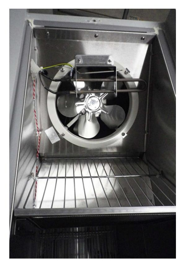
When you remove the cover, you will see the fan motor behind, with the heating element and temperature sensor attached to the front of it.
