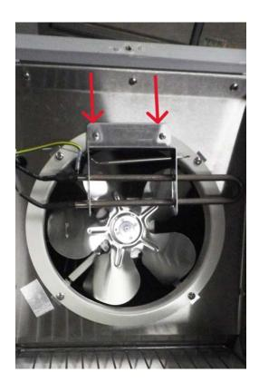
Once the fan motor and fan blade are in position, reattach the bracket containing the heating element and temperature sensor.
