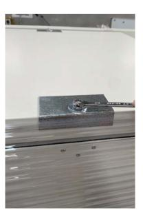
Using a 5mm allen key, unscrew the allen bolts that is holding the cover of the blanket warmer fan enclosure.
