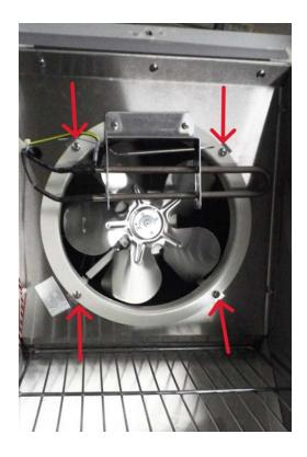
Please Note: Reattach the fan blades after fixing the motor into the shroud in the blanket warmer.
