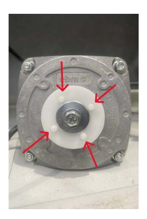
To reattach the fan blades, first remove the central screw cap in the middle of the motor. Then, place the fan blades over the four plastic locating pins on the central spindle. Once the fan blades are in place, screw the central screw cap back into place.
