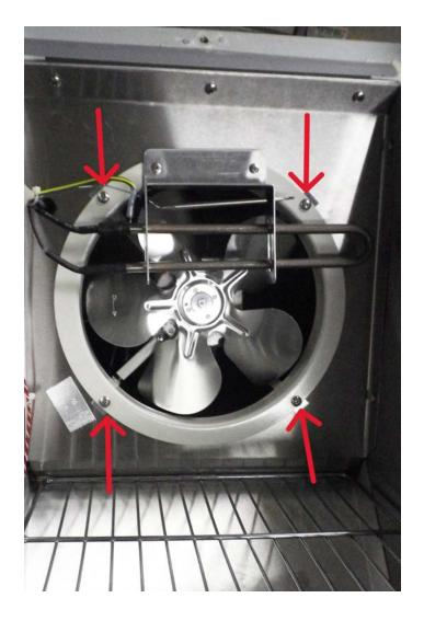
Once the fan blades have been removed, use a Phillips head screwdriver to take out the 4 screws securing the fan motor bracket inside the enclosure.
