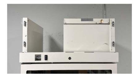
Pull the panel forward free of the blocks. This will allow you to access the enclosure that contains the evaporator fan
