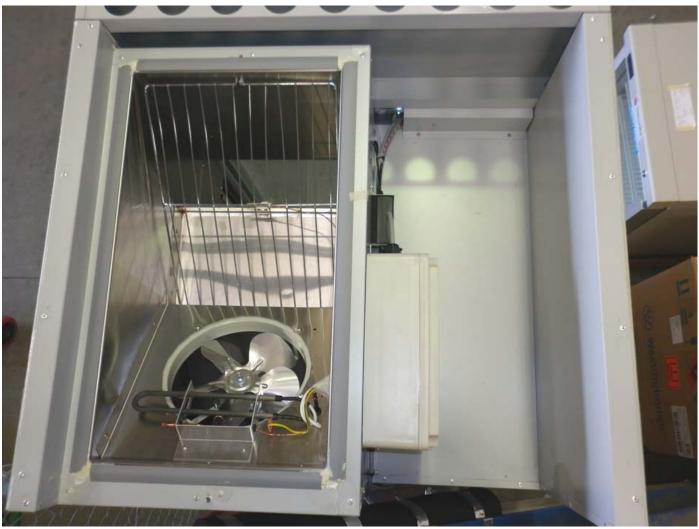
After removing the fixings, you might need to use a large flathead screwdriver to gently pry the cover upwards and remove the lid from the fan enclosure.
