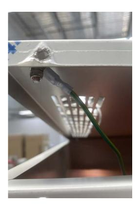
Once the Omron Controller has been installed, place the cover on top the oven and reattach the green and yellow earth wire to the spade clip to the spade terminal. Once the the earth wire has been connected, let the cover sit on to the oven and ensure that the screw holes of the cover are lined up with the cabinet. Screw the cover back into place.
