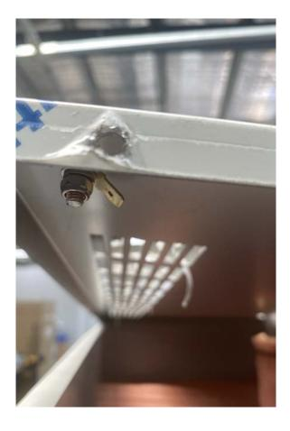
Once you unscrew these screws lift off the top cover and tilt it up. Located at the back of the oven cover on the underside (next to the rectangular vents) you will see a green and yellow earth wire connected via a spade clip. Remove this earth wire from the cover and then you will be able to remove cover. With the cover removed you will be able to access the Omron controller.
