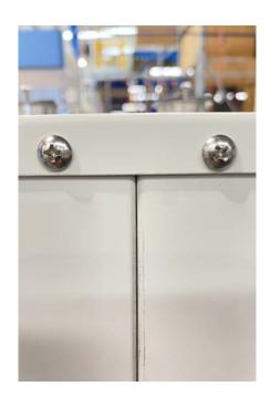
Unscrew the screws holding the top cover of the oven in place. There will be six in total; two on either side of the cabinet and two at the back of the cabinet.
