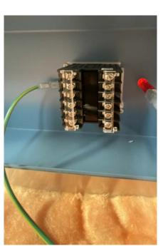
Disconnect the wires at the back of the controller, noting where each wire is located. Please note the included electrical diagram for wire connection locations.
