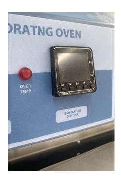
Slide the new controller into the front panel of the oven.
