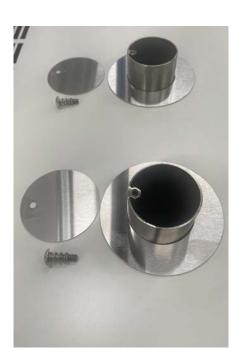
One top of the oven you you will see the oven exhaust and intake ports. Unscrew the screws holding the covers of the ports and remove them. **Please note:** Some lab ovens only have one port.
