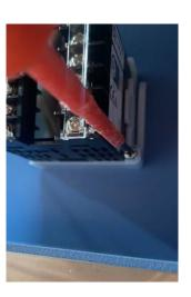
Replace the white fixing bracket and tighten the screws to hold the controller firmly in place.
