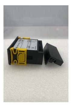
To access the wires at the rear of the ED3300 controller, remove the black the plate by pushing the locking tabs. This will disconnect the back plate and allow access to the screws holding all the wiring in place.
