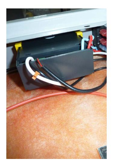
Once the wiring has been reattached the back plate can be replaced.
