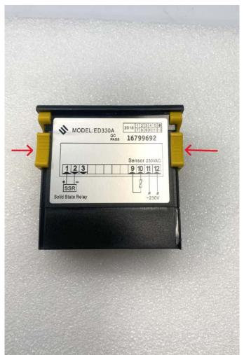
After removing all the wires, press the tabs inward on the yellow clips that hold the controller in place. This will allow the yellow clips to slide off the back of the controller. Once the clips are removed, the old controller can slide out of the front panel of the bath.
