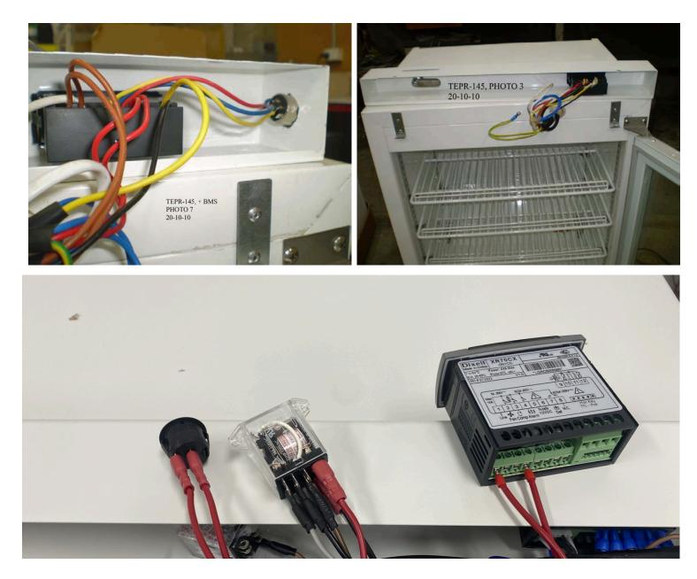
Access the the controller is possible by unclipping the bottom of the front panel of the 145 cabinet or undoing the three screws on the 200 cabinet. The electrical schematic on the following page gives details on the change over.
