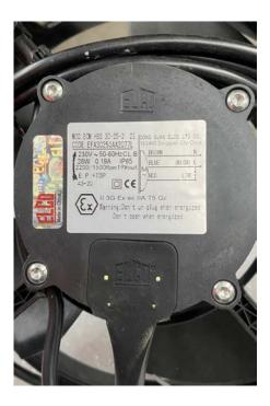
The Elco fan may be one of two different models that are used in the Climatron cabinets. One has a grey power cable and other one has a black power cable. Each has a different wiring configuration but in each instance the (low speed) red wire has to be added to the (high speed) brown or blue wire in the terminal block. This will slow the fan speed.
