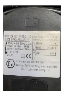
The Elco fan with the black wiring has the following wiring configurations:
