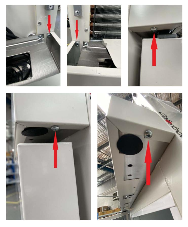
Remove the fascia panel containing the controller, lock, and door switch by undoing the screws in the top corners and along the bottom.
