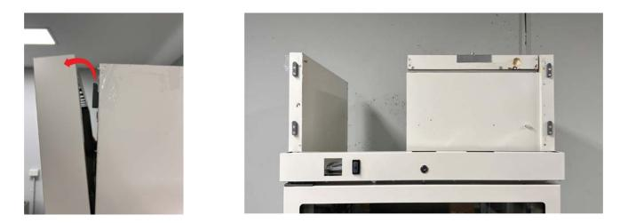
Pull the panel forward free of the blocks. This will allow you to access the lock and barrel
