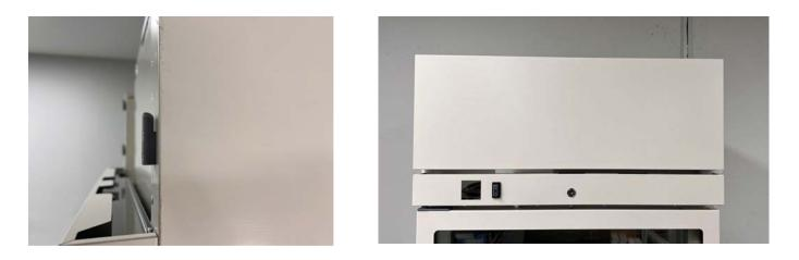
With the door switch and top panel in place, you can reinstall the front panel. Place the panel slightly above it's final position matching the rectangular holes with the locating blocks.
