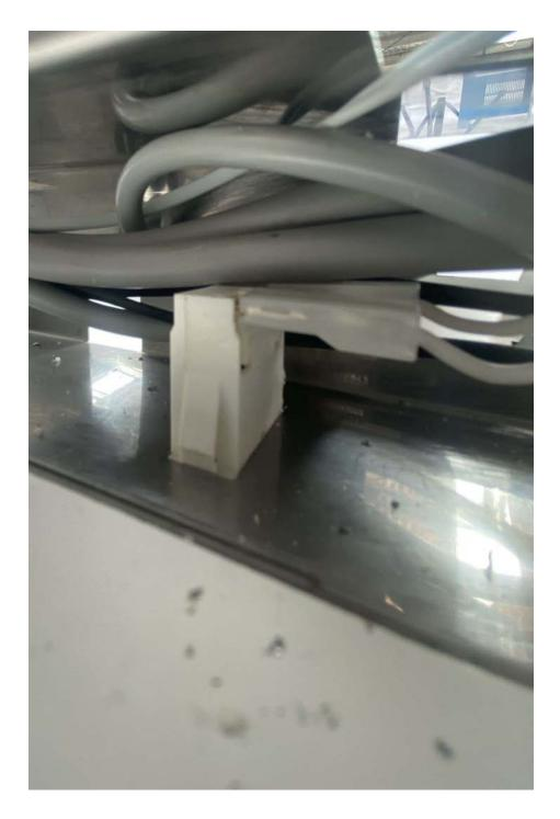
Once the door switch has been put in place, reconnect the spade connectors to the terminals.
