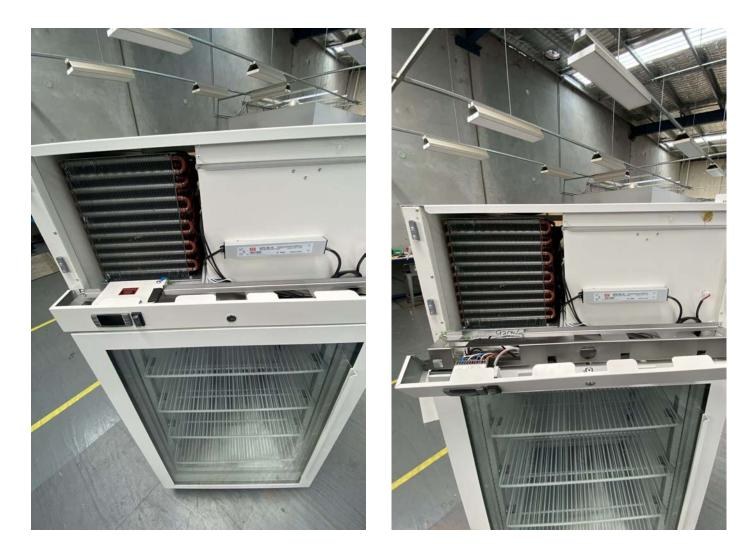
With the screws removed, carefully pull the fascial panel forward slowly to access the door switch in the centre of the fascia panel. The wires of the controller will hold the panel in place and stop it from falling.
