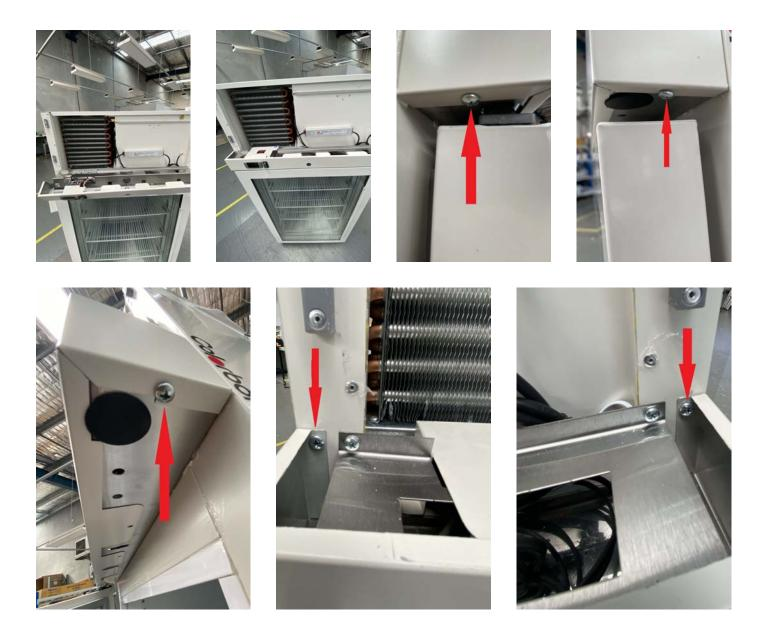
After reconnecting the door switch, reattach the front fascia panel using the screws removed earlier.
