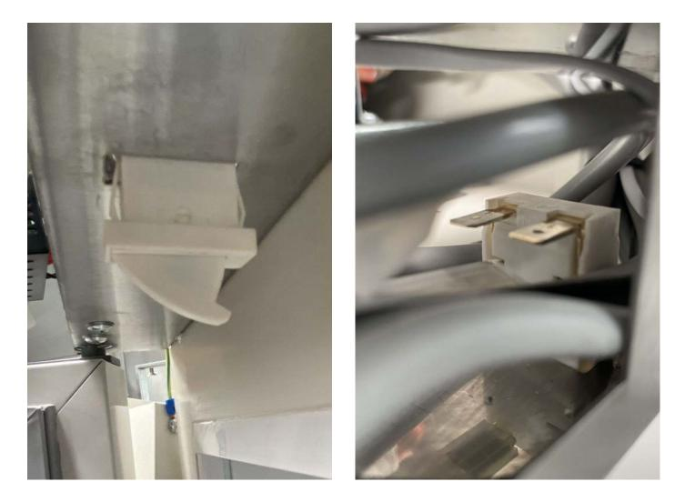
Take the new door switch and push it through the cut out ensuring that that the electrical pins are facing the left and side of the fridge. i.e. towards the Dixell controller
