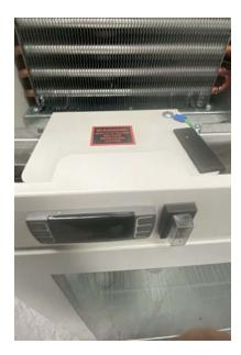
Once the panel is removed you will then see a metal plate covering the controller.
