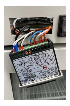
After removing the white clips, push the controller through the front panel to access the wires.
