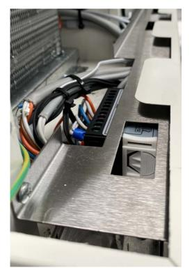
Once the controller is in the front panel, it can be fixed into place. Slide the white clips through the grooves on the side of the controller.
