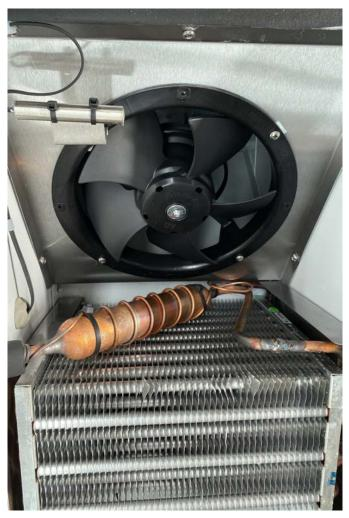
With the cover off, you will see the evaporator coil, the evaporator fan and the silver tube which contains the Dixell Hot Key sensor. The return air, Dixell sensor is on the other side of the evaporator and fixed to bracket against the wall (see the yellow circle).
