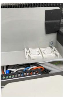
You will find two white fixing clips on either side of the controller. To unlatch the tabs of these clips, slightly push the white tabs of these clips inwards toward the controller. Then, you will be able to slide the clips off the back of the controller.
