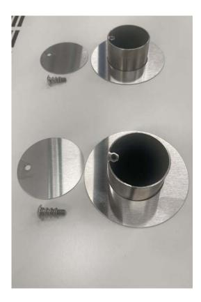
One top of the oven you you will see the oven exhaust and intake ports. Unscrew the two screws holding the covers of the ports and remove them. This will alow for the top of the oven to be removed.
