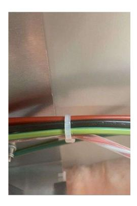
Reattach the wires of the PT100 sensor to the back of the controller and then cable tie the PT100 wire to the other wires inside the oven.
