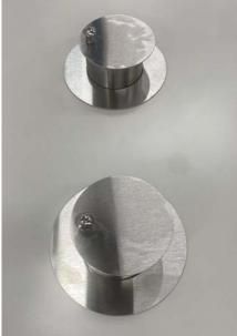
Screw the vent covers for the inlet and the exhaust port back on.
