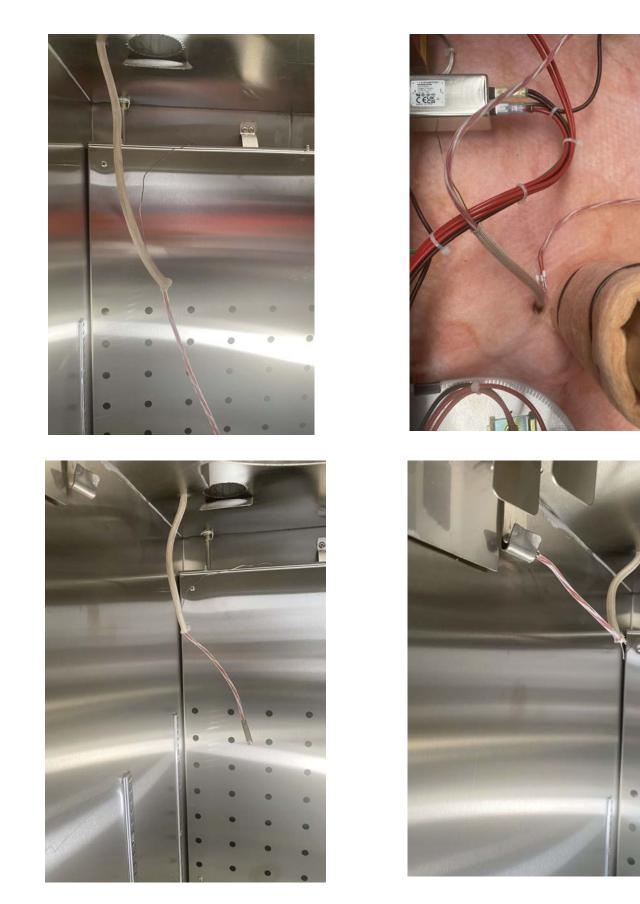
To install the sensor, insert its end into the white sheath hanging inside the oven and feed it through until it comes out at the top. Once the back end of the sensor is fed through, place the sensor bulb back into the metal support.
