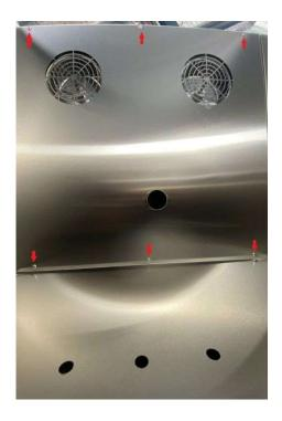
Slide the internal top panel back into place and fix it with the original six screws. You can then re-insert the shelvex clips at your required level and put the shelves back.
