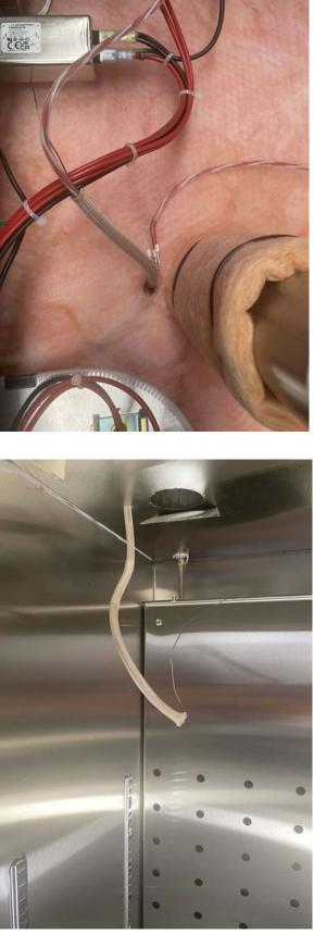
Once the head of the PT 100 sensor has been removed from the metal support, pull the PT100 sensor through the sheath from the head of the sensor and into the oven interior, until it has been pulled completely out.
