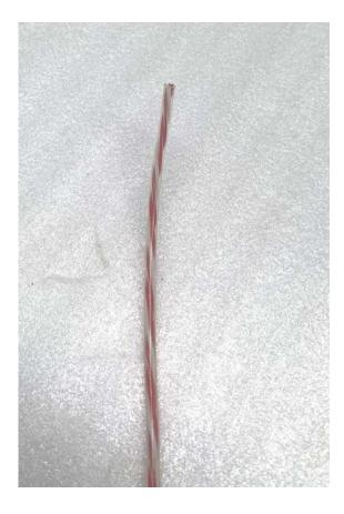
To make it easier to thread the sensor through the white sheath it is recommend that you evenly cut the three loose wires off while ensuring that the plastic casing is still wrapped around the wires.
