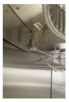
On the inside of the oven, the PT100 sensor can be located in at the top of the oven next to the blower wheel, resting in a curved metal support
