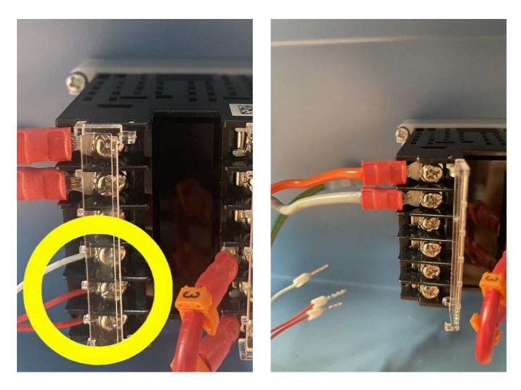
Undo the three sensor wires wires (2 Red and 1 White) at the back of the Omron controller
