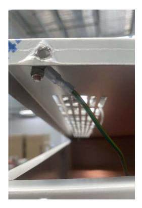
Once the Pt100 has been installed in the back of the controller, place the cover on top the oven and reattach the green and yellow earth wire to the spade clip to the spade terminal. Once the the earth wire has been connected, let the cover sit on to the oven and ensure that the screw holes of the cover are lined up with the cabinet. Replace the screws and fix the cover back into place.
