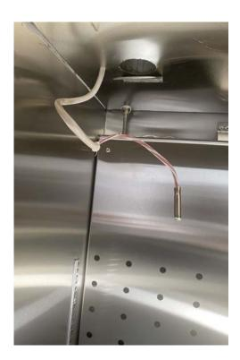
Generally to remove the PT100 Sensor from the curved metal support, all you will need to do is pull the sensor out. If the sensor is stuck, use a pair of pliers and bend the metal back slightly. This will allow the PT100 sensor to be removed.
