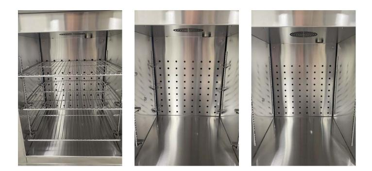
To the access the PT100 Sensor from inside the oven, first make sure the oven is cool and then remove the oven shelves and Shelvex clips
