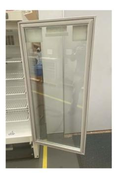
Slowly work your way around the door, removing the door seal from the groove until it is completely detached.
