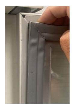
Open the fridge door and from the top corner, pinch the door seal and begin to peel it away.
