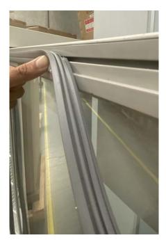
Start from the top corner of the fridge, firstly orientate the new seal to the door and then take the corner of the seal and push it into the groove of the door frame. Make sure the ridged side of the door seal is the side that is inserted into the groove.
