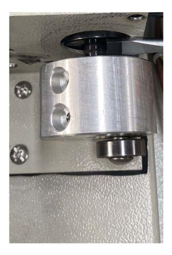
After removing the Allen keys, you can slide the front of the motor off the spindle. If the front of the motor is too tight, you can carefully loosen it by inserting a screwdriver between the front of the motor and the right angle bracket, and then lever it off.
