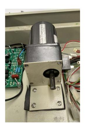
Remove the orange cap and the four black screws in the new motor. This will allow you to install the motor against the metal right angled bracket.
