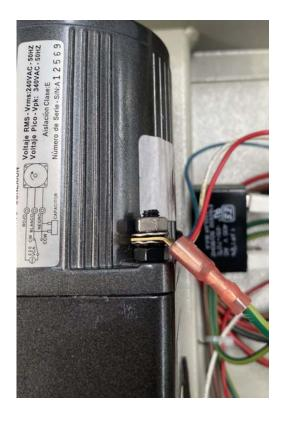
Reattach the earth wire to the motor and tighten.
