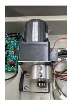
Using a 4mm Allen key remove the screws holding the head of the motor in place.
