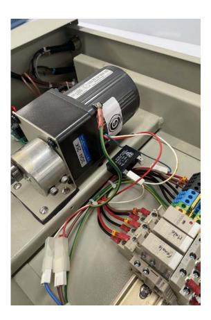
The motor provided to you has wires that are not yet connected. To get it working, you will need to attach crimp connectors to one end of the red and white wires. These wires will then fit into the black electrical block that is located next to the motor. As for the other wires, you will need to add BP connectors so that they can be connected to the black and blue wires.
