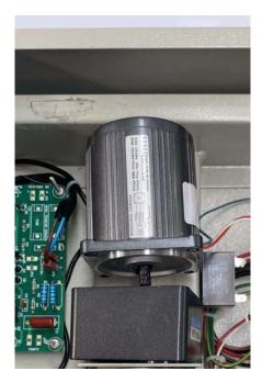
After removing the head of the motor, you can take out the rest of the motor by unscrewing the 4 black screws. Once you remove the screws, the motor will come apart, allowing you to take it out. Then, you can replace it with a new motor.
