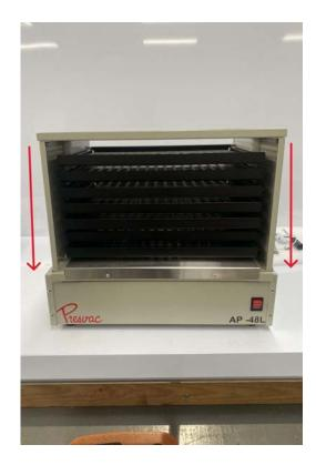
Lift the top shelving unit and put it back onto the base of the platelet shaker. Be sure to ensure that the white wheels of the shelving unit sit on rails in the base.
