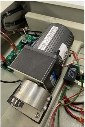
Disconnect the earth wire from the motor using an earth wire of similar
