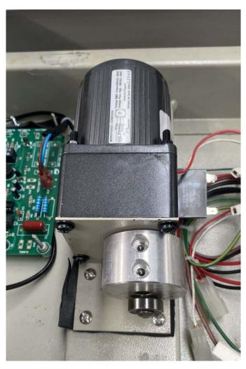
Make sure to slide the front part of the motor over the spindle, ensuring that the keyway of the spindle is facing upwards since this is where the screws will go into.
