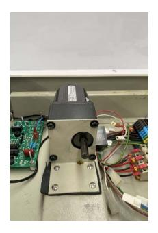
Fix the motor back in place with the four black screws.
