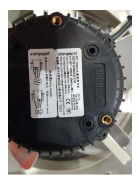
To install an older model fan in an older style cabinet, you'll need to splice the fan wires and chamber together, following the wiring instructions on the back of the fan.
