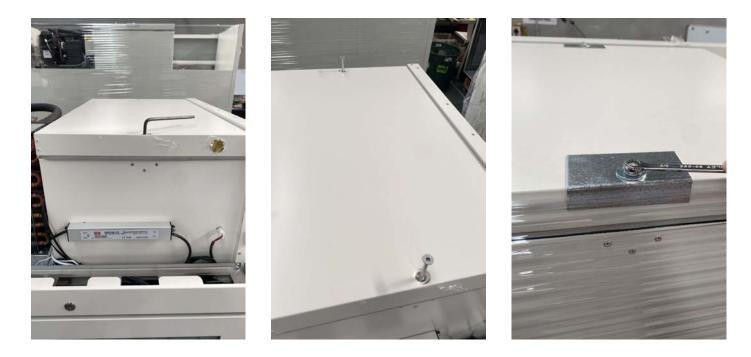
Using a 5mm allen key, unscrew the allen bolts that is holding the cover of the evaporator enclosure.
