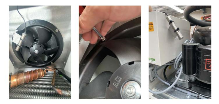
Use a small Philips head screwdriver to remove the Dixell hot key sensor housing and set it aside.
