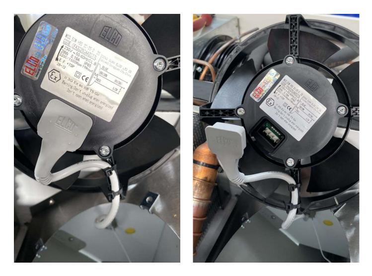
Disconnect the grey plug from the fan and cut the cable ties securing the fan power cable to it. This will enable you to swap it with a new fan.
