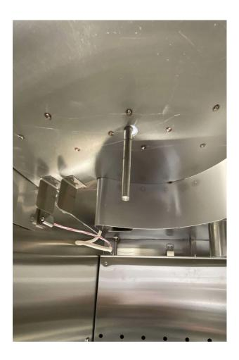
After loosening the grub screws, slide the blower wheel off the central fan motor shaft.
