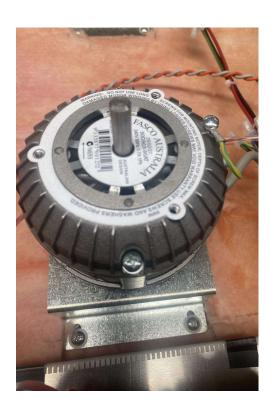
After fixing the motor to the top hat, reattach the top hat to its original position and secure it with the crews removed earlier.
