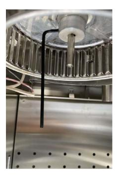
To detach the blower wheel from the D-Series motor, use a 3mm Allen key to loosen the grub screw that holds it onto the shaft. Be careful not to remove the screw entirely. There are two screws on either side of the fan motor shaft that you need to loosen.
