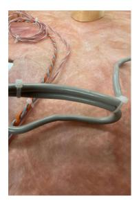
To separate the cables, remove any plastic cable ties that may be holding them together.
