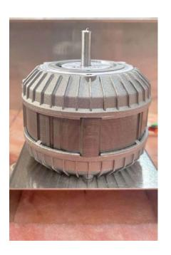
To remove the D-Series motor, first remove the cooling fan by sliding it upwards and off the top shaft.
