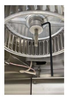
Use the 3mm Allen key to tighten both grub screws after positioning and aligning the blower wheel.
