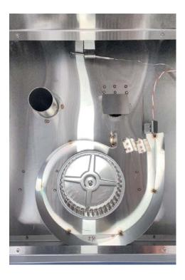
After removing the screws, carefully slide out the panel to avoid scratching the walls. Once removed, depending on the size oven, you will have either 1 or 2 the blower wheels in the roof of the oven will be visible.
