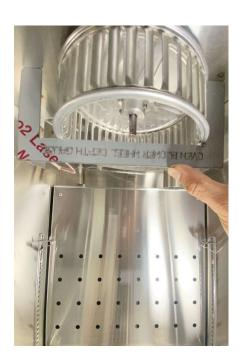
To reinstall the blower wheel, slide it back onto the shaft. Then, use the provided height guide to position its base correctly. Align the guide as shown above.
