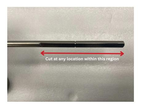
The Shaft can be cut with at any location indicated within the bounds of the arrow above to suit your cabinet. To cut the shaft you can use a hacksaw, angle grinder or any equivalent metal cutting tool.
