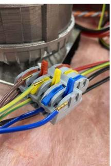
The D-Series motor can be connected to the main terminal block through a connector. To install the D-Series motor, follow the wires backwards from the motor to the connector and lift the tabs to free the wires. Once the tabs have been raised, gently pull out the wires.
