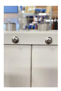
Remove the six screws holding the top cover of the oven in place; two on either side of the cabinet, and two at the back of the cabinet.
