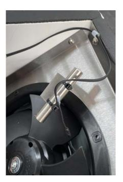
To remove the sensor, gently turn the silver tube 90 degrees. You will notice that the tube is filled with silicon. In most circumstances, the sensor can be easily pulled out of the tube after turning it. However, if the sensor proves to be difficult to remove, you can gently scrape the silicon from around the sensor to make it easier to remove.
