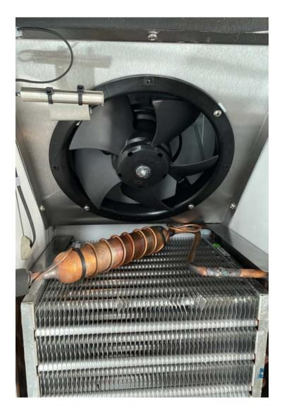
After removing the cover, you'll be able to see the evaporator coil, fan, and a silver tube containing the Dixell Hot Key sensor.
