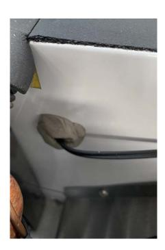
Thread the new Dixell Hot Key Sensor back into the section of the evaporator fan. Replace the putty once you are finished.
