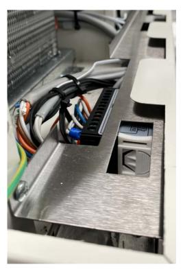
Once the hot key sensor is attached, the controller can be fixed into place. Slide the white clips through the grooves on the side of the controller.
