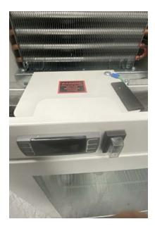
Once the panel is removed you will see a metal plate covering the controller.
