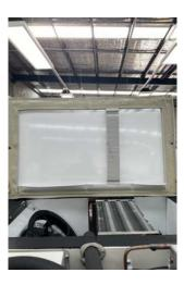
To open the evaporator enclosure, you need to take a large flat head screwdriver and insert it between the foam tape and the top of the enclosure. Then, you should gently lever the screwdriver upwards to break the seal. This will allow you to remove the lid from the evaporator enclosure with ease.
