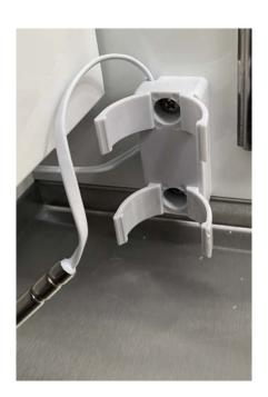
To remove the bottle sensor, first, unscrew the black cap from the bottle, and then slide the sensor through the black bottle cap. Once the sensor is out, use a Phillips head screwdriver to undo the two screws of the plastic bottle holder. This will enable you to slide the sensor through the back of the cabinet for replacement.
