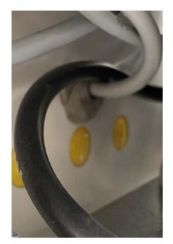
Insert the new sensor into the conduits of the evaporator enclosure, then seal the surrounding holes with the original putty.
