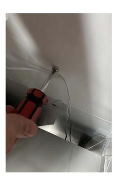
Drop the sensor down the back of the fridge and reattach it to the back wall with the fixing screw.
