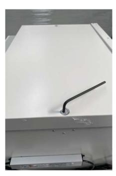
Install the evaporator enclosure lid. Make sure that the strip of foam going across the top is placed on top of the evaporator coil. This is to ensure that hot air is cooled through the evaporator rather then go above it. Once the lid is in place you can screw it down.
