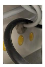
To remove the wire from the sensor against the back wall of the fridge, undo the fixing screw. Additionally, take off the putty around the conduit that the sensor wire passes through from the evaporator enclosure to the front of the fridge. However, make sure to keep the putty as you will need it later to seal the area around the new sensor.
