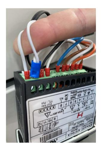
The bottle sensor, door switch and the return air sensor (Black NTC Dixell sensor) are connected in the same common terminal 11 via pin crimp connector. To remove this you have to cut the connector. Once you cut this wire, thread it through the conduits leading into the evaporator enclosure and then this will allow you to remove the bottle sensor completely. You will also have to remove the other wire from terminal 12.
