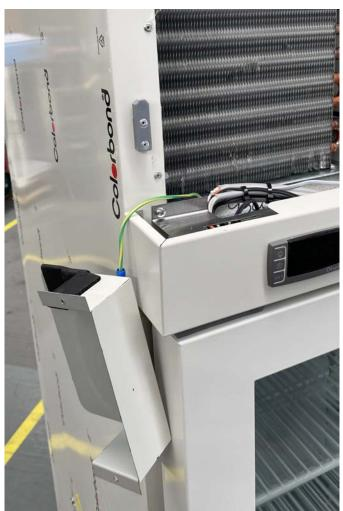
After removing the screws, lift the plate to reveal the controller. You can place the plate either behind the controller on the evaporator coil, or to the side.
