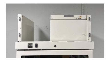
Pull the panel forward free of the blocks. This will allow you to access the controller
