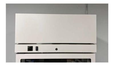
You can reinstall the front panel. Place the panel slightly above it's final position matching the rectangular holes with the locating blocks.
