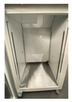
Remove the shelves and Shelvex clips. This will allow you to access to the bottle sensor and remove it.
