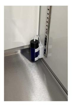
Screw the bottle housing over the sensor wire. Place the sensor through the black bottle cap and then place it into the bottle and screw the lid into place. Attach the bottle back into the bottlle housing.
