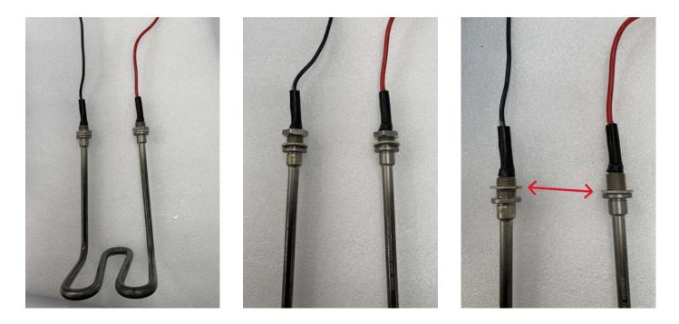
Before installing the new element, remove the nuts and foam washers. Discard the foam washers; the original metal washers used with the old element will take their place..
