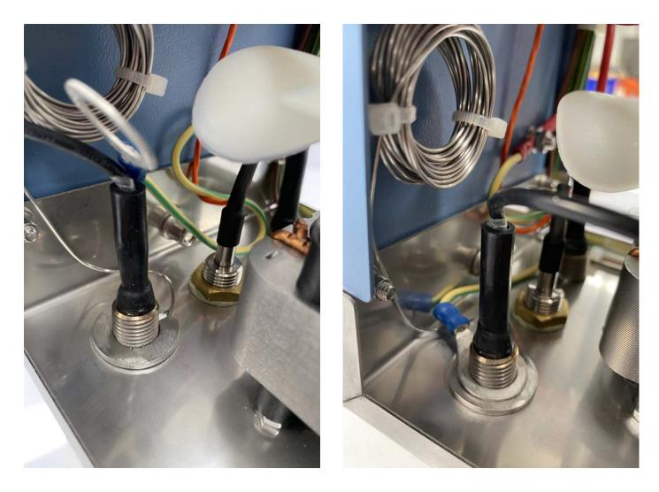
Slide the metal washer over the black wire. Please make sure that the wire for reset thermostat fits into the groove of the washer. Once in place thread the earth wire over the element wire.
