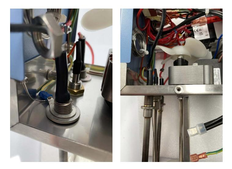
To remove the element from the Unistat housing, first locate the terminal connected to the black wire. Look for an earth wire looped around this terminal with a ring. To remove it, simply pass it over the end of the black wire. After this, you can safely pull the element out.
