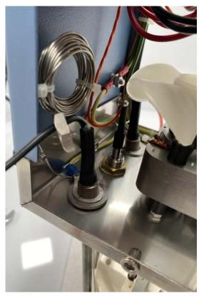
To remove the element, first loosen the nuts that are holding it in place.
