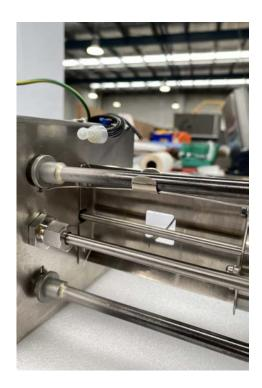
Before screwing the element in place, reattach the reset thermostat to the heating element via the metal fixing clips.
