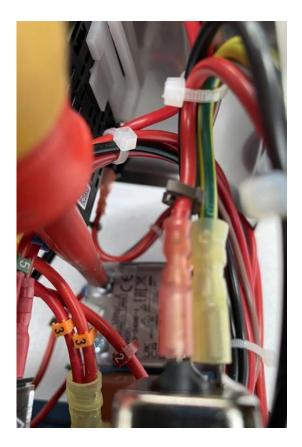
Follow the red wire from the heating element to the relay on the side wall. Unscrew this wire from the relay.
