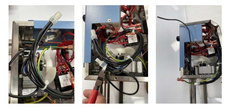
The black wire from the heating element is tied in with other non terminated wires at a BP Connector. Cut this BP connector off and you will then be able to separate and remove the black element wire fom this group of wires
