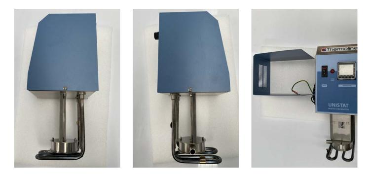
Unplug the Unistat from power and lay the unit flat. Undo the screws on either side of the Unistat cover. Once the screws are taken out, the cover can be carefully removed. The cover is connected to the body of the Unistat with an earth wire via a spade clip. Pull this earth wire from the spade clip. You can then put the cover to one side.
