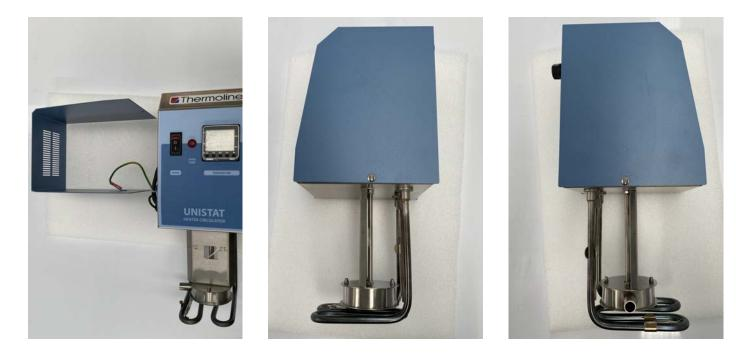
Reconnect the earth wire to the cover of the Unistat. Put the cover back in place it on the Unistat and reinsert the screws.
