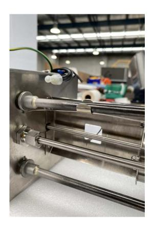
To disconnect the reset thermostat from the element, you need to remove the metal fixing clips.
