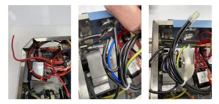
For the red wire from the element, using a wire stripper remove the red sheath and then screw this back into the real.
