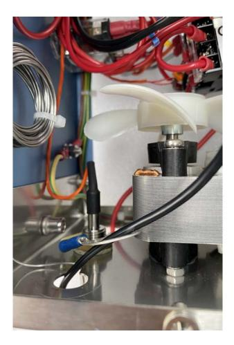
Thread the wires of the new element into the Unistat housing.
