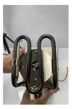
Once tightened, look down along the length of the Unistat. You will notice the element is slightly crooked. You can straighten this, by gripping the end of the element and twisting it with your hand to straighten it up.
