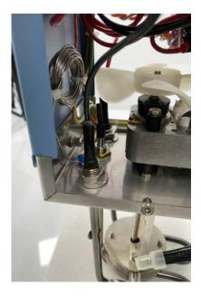
Place the nuts over the wires and tighten
