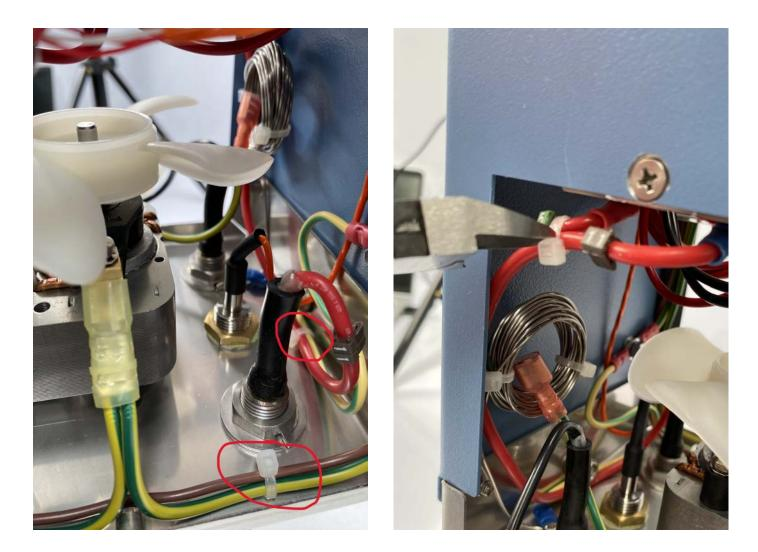
Using a wire cutter or similar cutting tool, remove the cable ties that are holding the wires together from the heating element.
