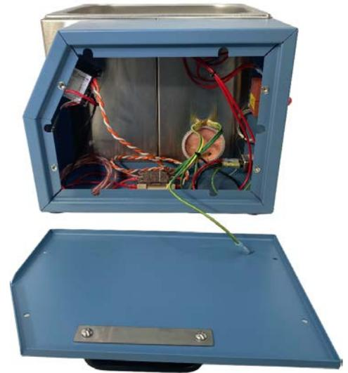
Unscrew the screws on the blue side of the bath electrical box.
