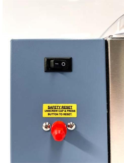
Push the switch through the hole in the electrical box. Be sure to note that "O" is closest to the bath.
