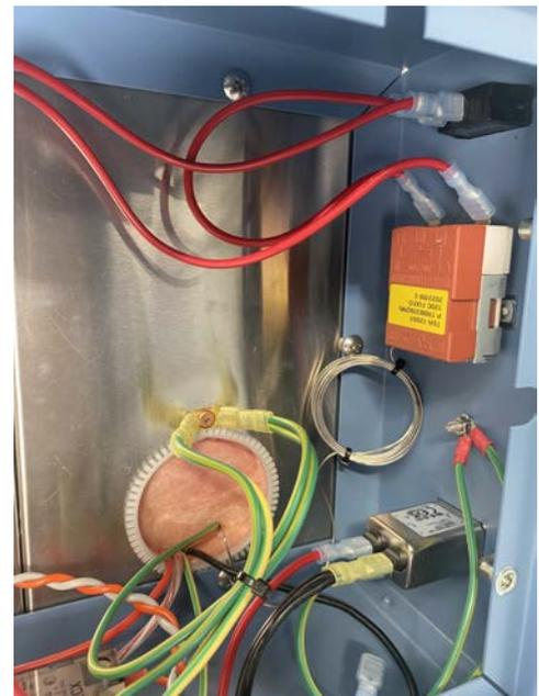
Once the switch has been inserted into the electrical box, reconnect the wires to the back of the new switch.
