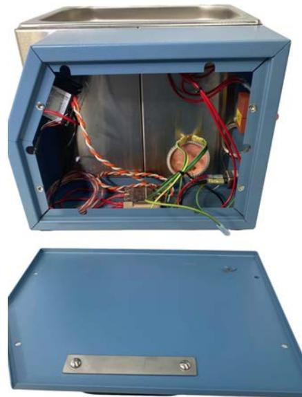
Once the side panel is open, disconnect the earth wire to completely remove the panel.
