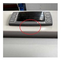
The faceplate is unclipped from the bottom via the small indent.
