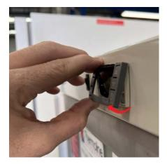
Once unclipped, pull the face plate out from the bottom and lift up to remove.
