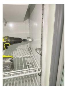
Once the tip of the hole saw reaches the internal skin of the cabinet, remove the hole saw and then use the hole saw to drill from the inside.
