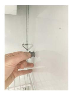
Insert the plastic bushes with the silicone bead on the outside and then the inside of of the cabinet. The orientation of long and short plastic bushes (inside or outside) doesn't matter as long as one of each is used to make the port hole.
